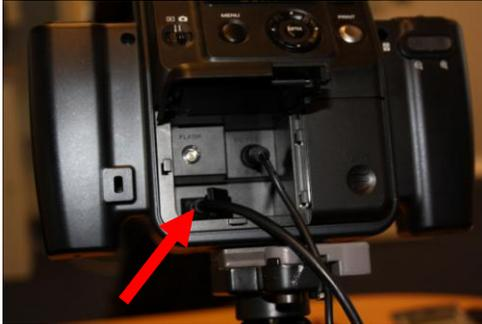
The USB cable may be connected to the camera at all times.
